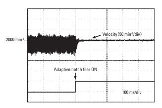
Fig. 4: Suppression of machine resonance with an adaptive notch filter
