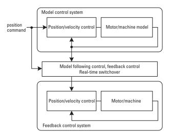
Fig. 3: Real-time switchover function for model following control and feedback control
